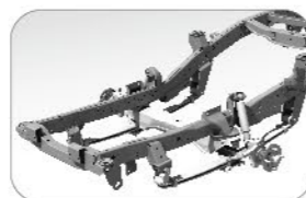
DURABLE RIGID FRONT LEAF SPRING SUSPENSION
